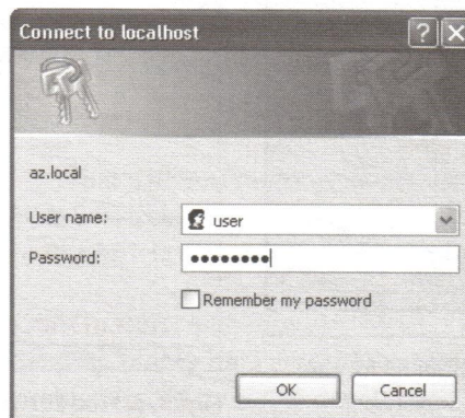
Figure 3. Basic Authentication challenge (as seen in the browser when testing the Web Service).
